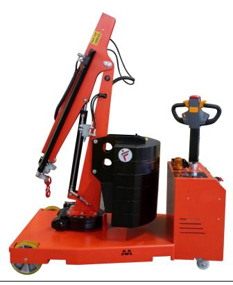
Our model FLEX G1000DB is a full electric powered counterbalanced mobile swivel crane with a lifting capacity up to 1 ton. One of the key features of this pick and carry crane is that there are no lateral outriggers, therefore this crane grants max mobility with suspended load. It is equipped with AGM batteries that can be recharged in areas with limited ventilation.
